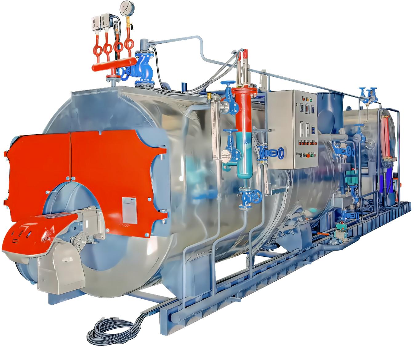
It is manufactured as a package unit and it contains all necessary devices and control equipment for steam production. It produces heat energy in a noticeably short time thanks to specially designed boilers. It can also be easily moved around on its steel chassis and used anywhere as plumbing, chimney and electrical connections are integrated in steel structure. As a result, it occupies less space and installation and maintenance are made easy.
