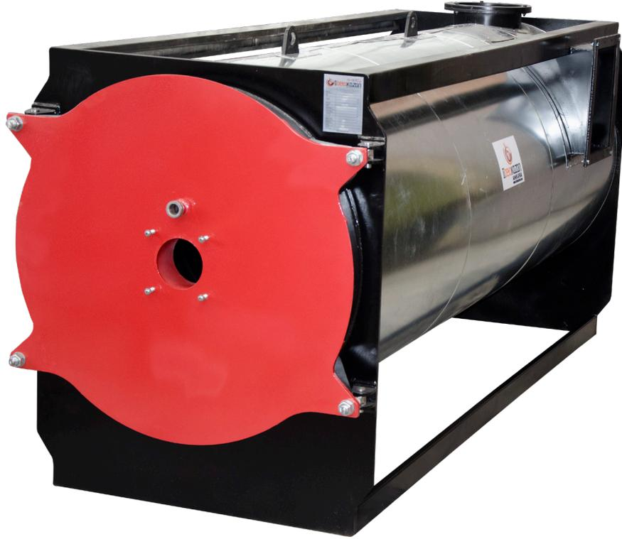
HAG series hot air boilers can be designed vertically or horizontally in accordance with standard or process-specific applications. These systems, designed for direct and indirect heating types, are extremely efficient. Direct heating system is used in applications where high temperature drying is required, and indirect systems are used in systems where fresh air is required for drying.
