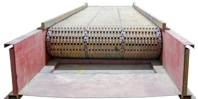
The coal must completely burn at the end of the grate. The ash of the coal that has completed its combustion is discharged from the end of the grate with an appropriate ash removal system. After discharging the coal, it returns under the combustion zone, and cools down since it is not exposed to combustion. As a result, the grate does not experience considerable thermal deformation as it is not exposed to elevated temperatures.
